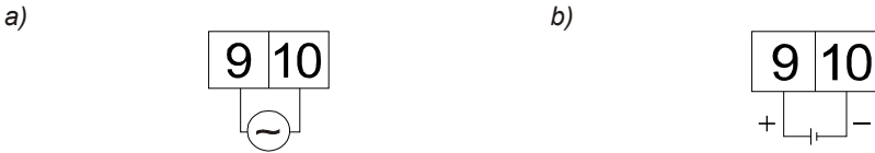
Figure 4.4. Connection of power source: a) supply 100 - 240V AC, b) supply 12 - 24V DC
