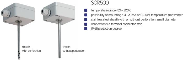
Resistance thermometers SCR500 are designed for ambient temperature measurement. There is a possibility of assembling a programmable temperature transmitter with a 4...20mA output signal into the housing. The protection tube with perforation allows for quick and precise temperature measurement, thanks to direct contact of thermometric resistor with ambient temperature.
