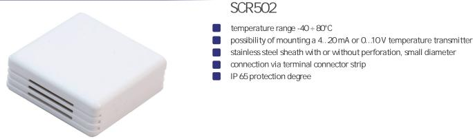
Resistance thermometers SCR502 are designed for ambient temperature measurement inside residential, office and industrial spaces. There is possibility of assembling programmable temperature transmitter with 4...20 mA or 0...10V output signal into housing. The housing with perforation ensures quick and accurate measurement. The interesting appearance of the sensor allows for installation in residential houses, ensuring appropriate aesthetics.
