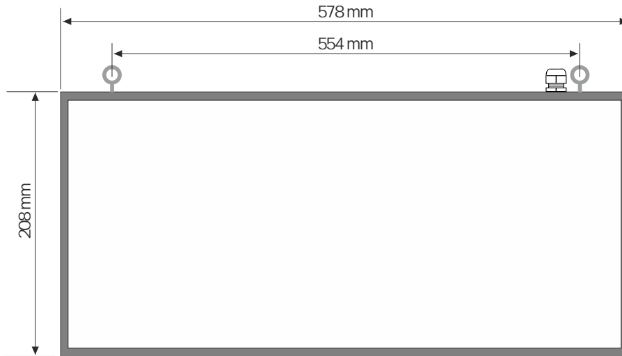
Case dimensions and distances between mounting holes
