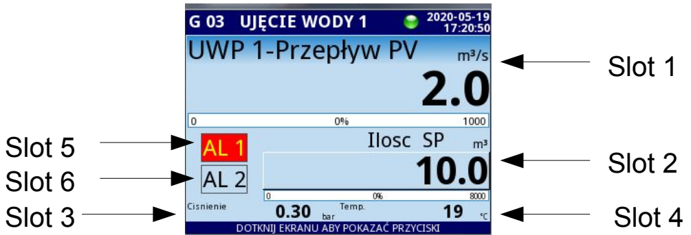
Fig. 7.160. Slots layout in controllers view
