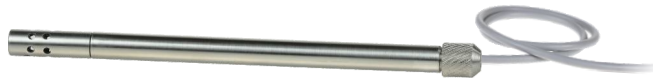
PPO-622-XX-X-X Cable probe Ø12, L=300mm, housing SS 316L, filter from SS mesh 25 µm
