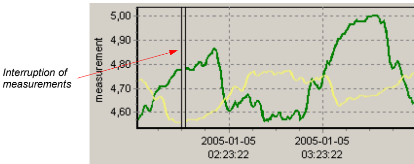
Fig. 3.11. Vertical lines on the graph - interruption of measurements
