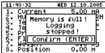
Fig. 7.15. Warning in “until full” recording mode
